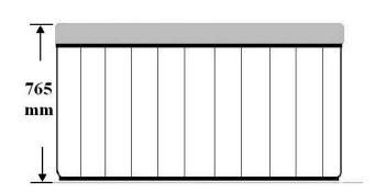
The **Plug 'n Spa** is manufactured to a height of 765 mm. It is designed to be set down on a firm flat surface and not set into the ground or a deck.
