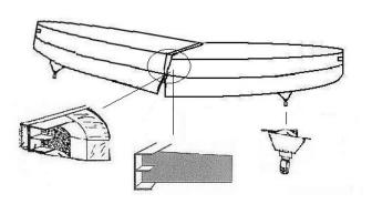
The cross section of the **cover** shows the insulating foam billets fitted with the rigid E bar for strength. Four evenly spaced lockable catches are fitted.
